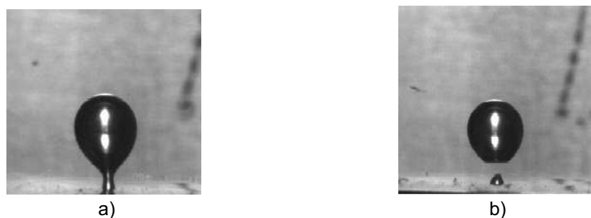
a) Bubble just prior to detachment b) Bubble just after detachment Fig. 2. Bubble detachment from a cavity of 0.6 mm in diameter for Re = 499 and Ja = 24 .
